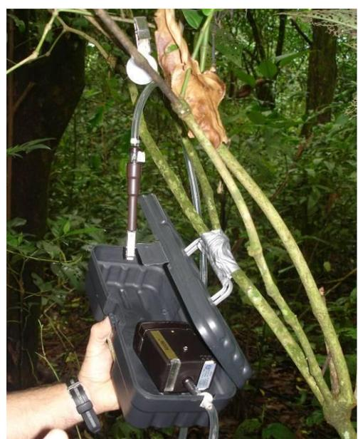
Figure 2: Active sampler hanging in a tree. The denuder was located at about 1.60 m height.
